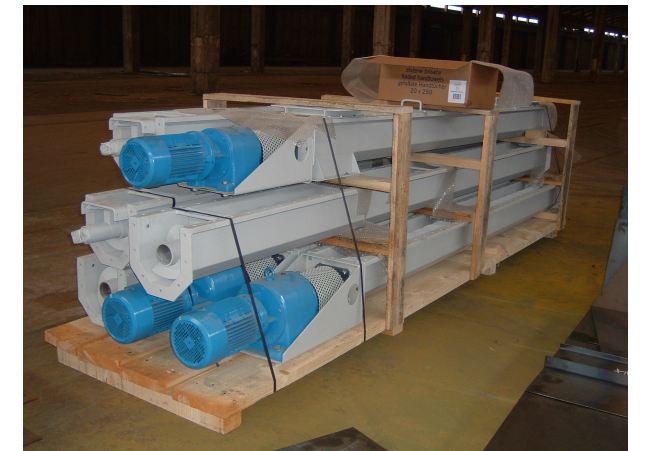
Screw feeder Ø200 mm
