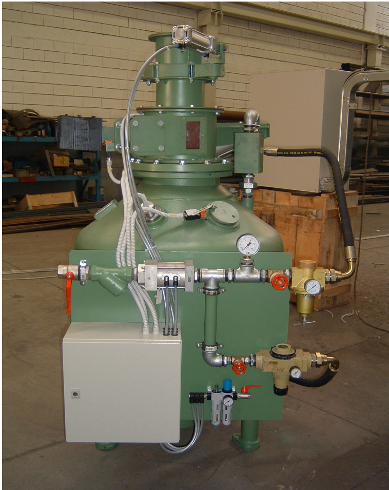
Pneumatic vessel 250 l with equipment
