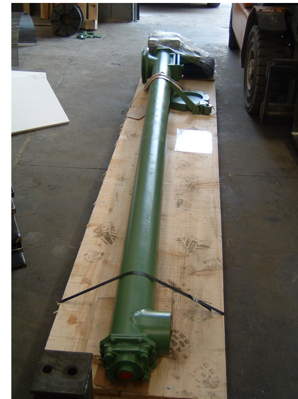
Screw feeder Ø150 mm
