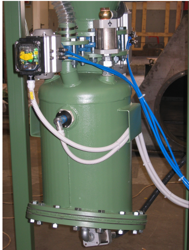
Additives pneumatic transport
